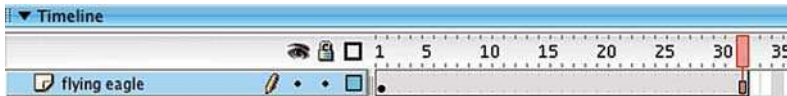
The Flying Eagle Layer lasts for 32 Frames. Therefore, the Animation will Loop Twice
